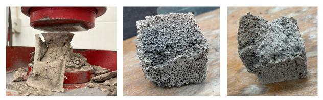
Figure 17. Specimens after residual compressive strength test: Lime.m (left), EPS.m (middle), Aero.m (right)
