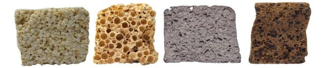
Figure 23. Zoomed photos. From left to right: initial EPS.m, post-heating EPS.m, initial Aero.m, post-heating Aero.m
