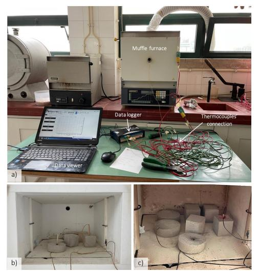
Figure 12. Test setup: a) general view; Specimens' placement post heating b) Lime.m and c) EPS.m and Aero.m
